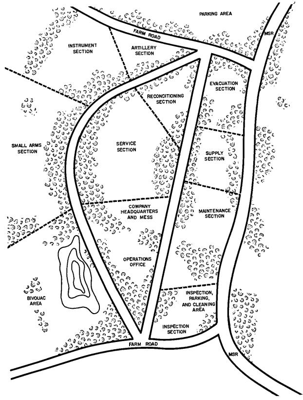
Figure 4. Sample layout of a general support company.
